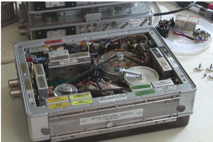
The inner workings of one of 3 Stellavox SM8’s
