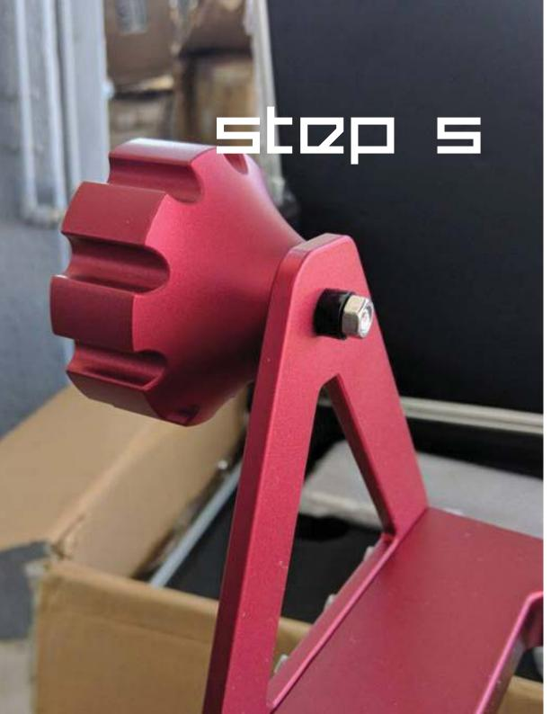
use the plastic bush provided as a spacer to connect the tourbillon to the stand, when you tighten the knob, it squeezes the plastic spacer and locks it into position.
